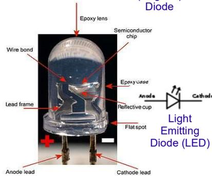
Can be used as LEDs to generate light
